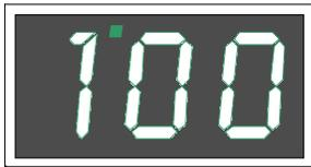
The Preset Display shows 3 alphanumeric characters that correspond to the current preset number, whether it's presently loaded or not. When the Preset Display is flashing a preset number, it is because you have entered Store mode and pressing the Store button will overwrite the current preset number's contents.
