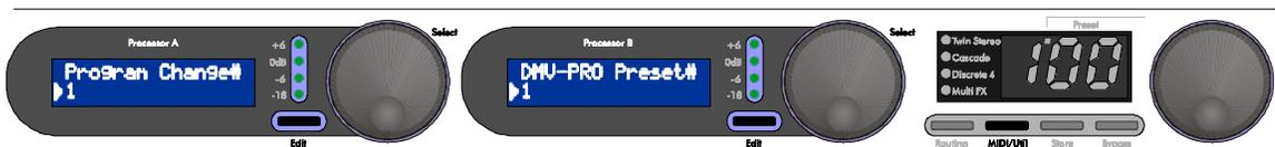
Next, turn Encoder (A) to select an incoming MIDI program change number that you wish to map. This control's range is from 1 to 128. Turn Encoder (B) to set the corresponding DMV-PRO preset number that will be recalled when the program change number in LCD (A) is received. The range of DMV-PRO preset numbers is from 1 to 100, or OFF to disable a program change number from recalling any DMV-PRO preset. Repeat this process to map other program changes.
