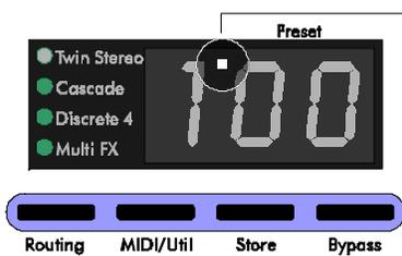
This light indicates that the preset you are looking at is not currently loaded and, therefore, will not match what you are hearing. Press the Preset Encoder to load (and hear) a new preset.
