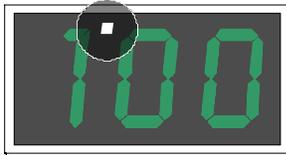
When you turn the Preset Encoder to view presets, the DMV-PRO's sound won't change until you press the Preset Encoder to load the preset. The Unloaded Preset Indicator is a reminder that you are viewing an unloaded preset.
