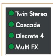
The DMV-PRO has four signal-routing options: Twin Stereo, Cascade, Discrete 4, and Multi FX. For a description and diagram of each routing, see page 26. Routings are selected by repeatedly pressing the Routing button (see the above Routing Button paragraph).
