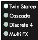
By editing any preset's routing, you are essentially building a new preset from scratch. When routings are changed, the DMV-PRO reconfigures its internal architecture and loads in default effects. The preset's former effects, class, and parameter values are all replaced.
