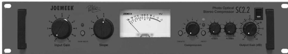
**INPUT GAIN** sets the audio gain of the stereo compressor. It's calibrated 1 to 11. With the control set at number 5, the gain through the compressor is about 0dB (no gain). With the control at maximum, the gain is about 20dB.
