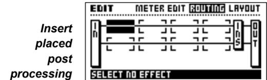
With this parameter you select if you want to have the Insert block present in the Routing grid, and if it should be placed before (Pre) or after (Post) the processing blocks.
